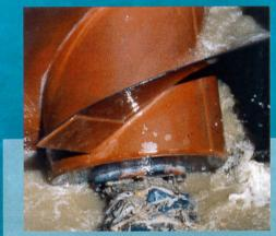
**Archimedes screws**Water lubricated bottom bearings.
