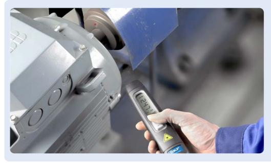
The laser optical system allows easy and quick measurements at a safe distance from rotating machinery.
