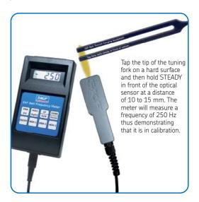
Results within  $\pm 1\%$  are acceptable. There is no adjustment possible. If greater variance is experienced, the meter should be returned for calibration. See section 7.2 for manufacturer's contact information.
