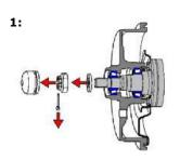
Remove the dust cover (either pressed in or screwed on), remove the split pin (if fitted). Remove the locking nut (ensuring that the correct rotation is noted) and flat washer. Place components in a suitable container for cleaning. Components should not be mixed with other components from the opposite side of the vehicle.
