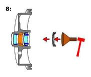
Install the inner bearing cone using the correct installation tool. Unwrap the seal from its protected packaging and install using the correct seal installation tool. Check to see if seal is fully seated into the drum/hub. Apply a 'LIGHT' smear of grease on the seal lip to reduce friction upon start up.
