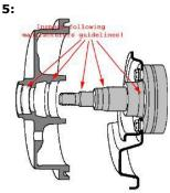
Clean and inspect all machined matching surfaces against vehicle manufacturers guidelines. If tolerances are exceeded, the drum/hub should be replaced.
