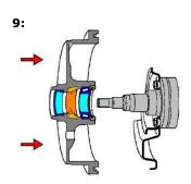
Apply 'Anti-fretting' paste (SKF-LGAF1) to the matching machined surfaces of the bearing and hub spindle. Carefully guide the drum/hub unit onto the spindle. Take care not to damage the seal during this procedure!
