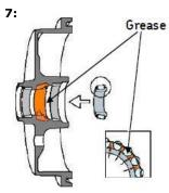
Using high quality CLEAN grease, fill the drum/hub cavity between the bearing seats, with the correct amount as per vehicle manufacturers guidelines. Do not overfill! Pack the bearing assembly, ensuring that the cone, bearing elements and the cage are completely impregnated with grease. Care should be taken at this stage, as dirt and grit could be pressed into the assembly!
