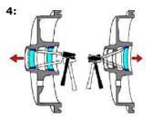
Wearing suitable eye protection, remove the inner and outer bearing cups using a brass drift and hammer. CARE MUST BE TAKEN that damage does not occur to the inner dimensions of the drum/hub unit!
