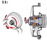
Lightly tighten locking nut by hand ensuring that the bearing elements are aligned. Whilst rotating the drum/hub, secure the completed assembly onto the spindle. DO NOT OVER TIGHTEN, as damage will occur to the rolling elements, cage, cup and cone!
