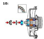
Following the same procedure as with the inner bearing assembly, use high quality CLEAN grease. Pack the bearing assembly, ensuring that the cone, bearing elements and the cage are completely impregnated with grease. Care should be taken at this stage, as dirt and grit could be pressed into the assembly! Install the bearing cone assembly, flat washer and locking nut.
