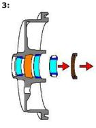
Remove the seal and the inner cone, once again ensuring that the rolling elements are protected from damage.
