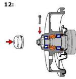
Use a 12" adjustable spanner to tighten adjusting nut while turning drum/hub. When drum/hub binds slightly, all parts are properly seated. Back nut off 1/6 to 1/4 of a turn or sufficient enough to allow 0.001" to 0.007" end play. Secure locking nut with a new split pin (if fitted). Place a little grease into the dust cap to deter corrosion from moisture and carefully install into the drum/hub unit.
