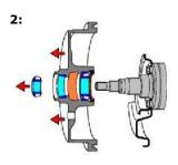
Remove bearing cone and place it in a clean cloth for inspection later, the bearing assembly (cup & cone) should not be stored with the locking nut, washer and dust cover, as damage could occur to the rolling elements.
