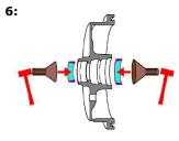
Install the **new** bearing cups into the drum/hub. Bearing components should not be removed from their protective packaging until just before installation. This reduces the chance of contamination from grit, dust and moisture which could seriously reduce the bearing life! Close inspection, using feeler gauges should be carried out to ensure that the cups are fully seated and not misaligned into the drum/hub bore.
