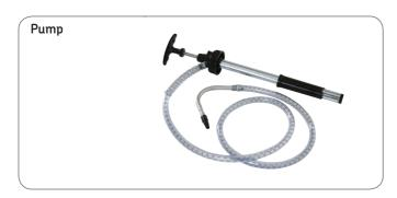
Suitable for viscosities up to ISO VG 680, AGMA grades 6-8, or SAE 140. Match with utility lids, making it suitable for 3, 5 or 10 litre drums (0.8, 1.3 or 2.6 US Gal). Provides high flow (aprox. 14 strokes per litre/US quart) and comes equipped with a long discharge hose of 1,5 m (4.9  $\,$ ft) and an anti-drip nozzle. If a smaller outlet is required, a reducer nozzle is available.
